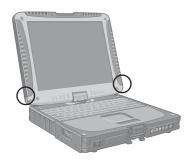
The tether can be attached to the bottom right or bottom left corner of the display. It prevents the pen (included) from falling accidentally.
